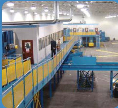
Single line MRF processing 17 tons per hour dry recyclables excluding glass.
