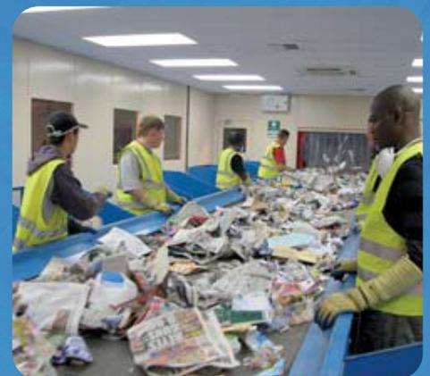
Pre sorting cabin within MRF. Cabins include air conditioning, fresh air intake, heating and lighting.
