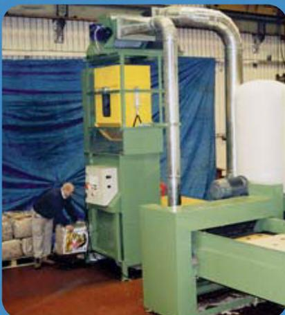
Complete animal bedding system including shredder, pneumatic feed and dust extraction, weigh hopper and bagging unit.
