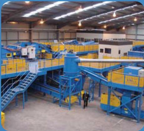
Recent installation 2006, processes 15 tons per hour of dry recyclables including glass.
