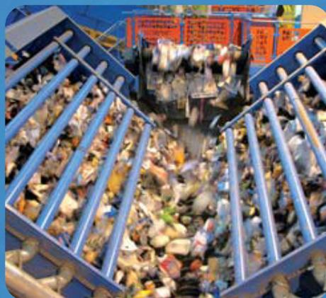
V-Screen disc screen separator within MRF. Capacity to separate/process up to 20 tons per hour dry recyclables.
