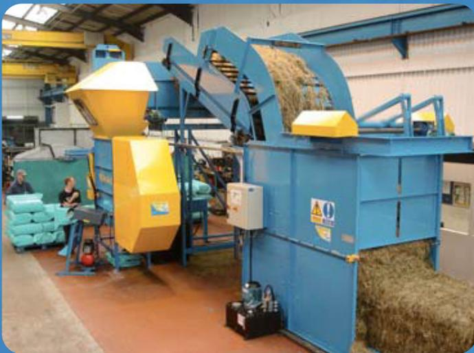
Haylage packing system including bale breaker, weigh conveyor and bagging machine. Finish pack weight 20kg.
