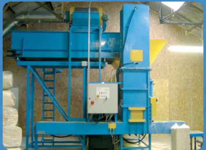
Dust extraction, weight conveyor and bagging plant (20kg).
