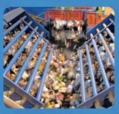
V-Screen disc screen separator within MRF. Capacity to separate/process up to 20 tons per hour dry recyclables.
