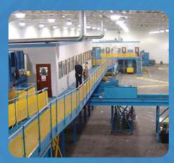
Single line MRF processing 17 tons per hour dry recyclables excluding glass.
