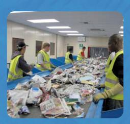
Pre sorting cabin within MRF. Cabins include air conditioning, fresh air intake, heating and lighting.
